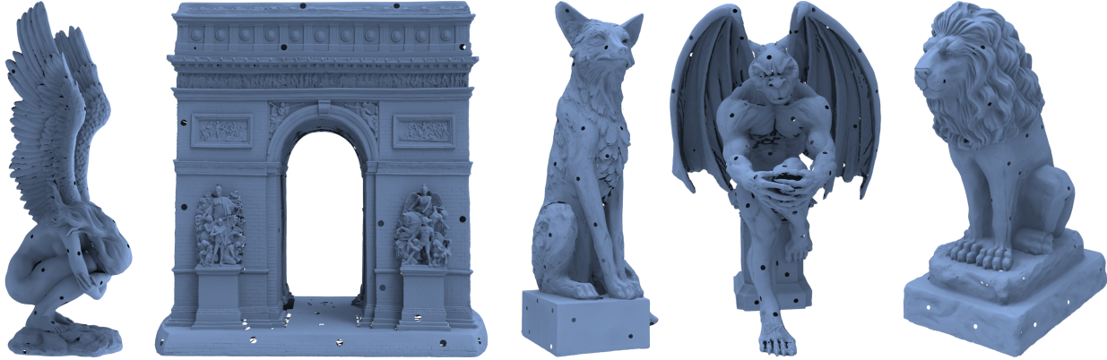
Figure 3. Ground truth models acquired using an industrial 3D scanner. From left to right: angel, arch, fox, gargoyle, and lion.
