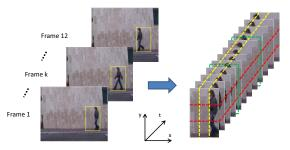
Figure 3. Example of computing HOG3D features for root filter. Left: 12 consecutive frames consisting one cycle of walking (annotations in yellow). Right: spatial area corresponding to the bounding volume, which (for this action type) is divided into 3 cells in x (yellow), 3 cells in y (red), 3 cells in t (green) to compute the HOG3D features for the root filter. The resulting feature descriptor is a  $3\times3\times3\times20$  vector. (Part filters not shown here.)
