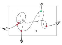
Figure 3. Fast winding number computation. Draw an arbitrary path to outside of the image frame, the winding number of a point equals the number of edges crossing from right (red dot) minus the number of edges crossing from the left (green dot).
