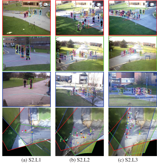
Figure 3: Tracking results on PETS 2009 for three cameras and ground plane; (a) low density (S2.L1, camera 1+5+7), (b) medium density (S2.L2, camera 1+2+3), (c) high density (S2.L3, camera 1+2+4); solid box: detected in this camera; dotted box: reconstructed from other camera; dashed box: interpolated (detected in no camera).
