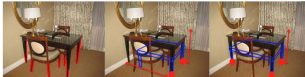
Figure 6. We use detected “pegs” to propose furniture with legs (left). Proposing a table from two pegs (middle) requires estimating the width/length and the height of the table, proposing it from three only leaves the height as a free parameter. View in color.
